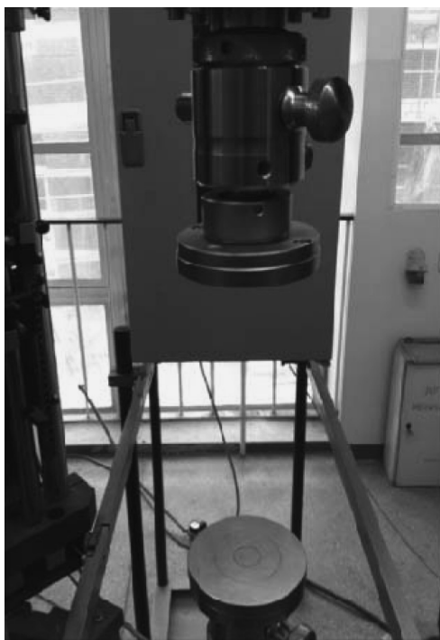
Figure 4. Specimen grips used during static compression tests
