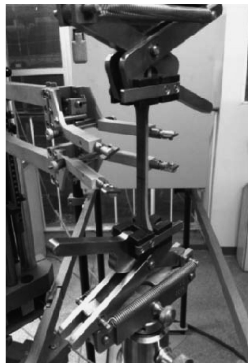
Figure 6. Dumbbell elastomeric specimen subjected to static tension
