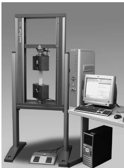
Figure 1. Zwick/Roell Z020 universal testing machine
