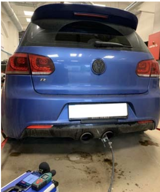
Figure 2. Orientation of recording microphone Source: authors.
